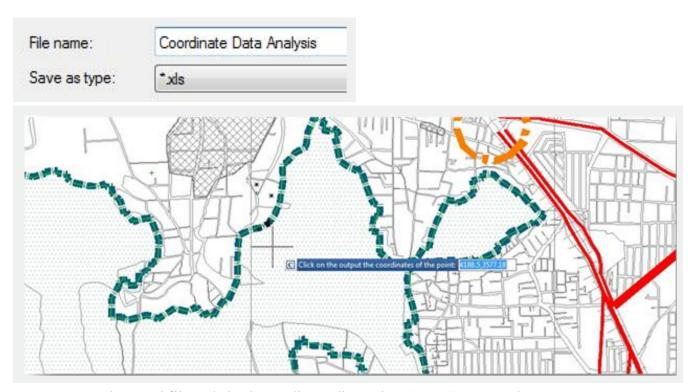
You can open the saved file and check out all coordinate data (X,Y,Z) extracted.
