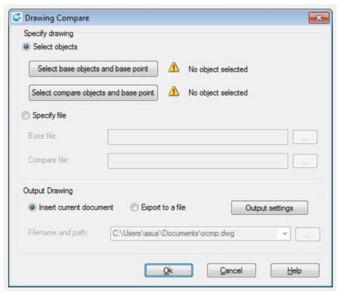
You can invoke the Graphic Compare dialog box by tipping OCMP command at command line or by dynamic input.
